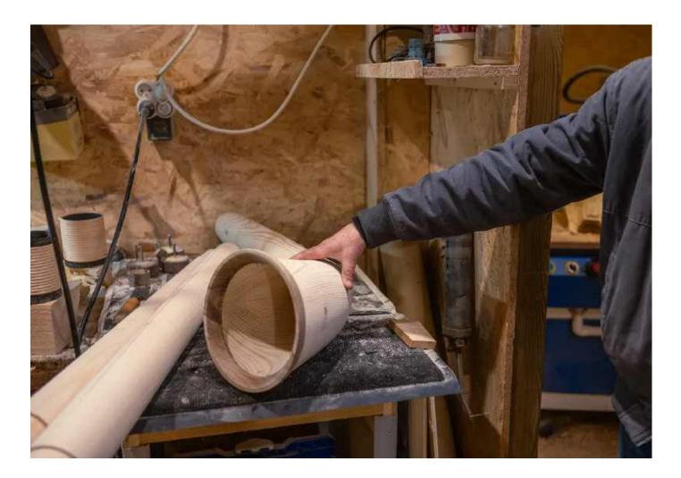
Although pretty and uniform, the instrument's symmetry goes beyond aesthetic appeal: It ensures that the wood's density is the same on both sides of the alphorn, leading to better sound quality.
